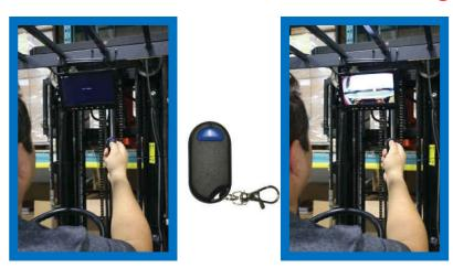
The key fob function allows the operator to only use the Eagleye when needed. Monitor view automatically turns off after 5 mins of inactivity.
