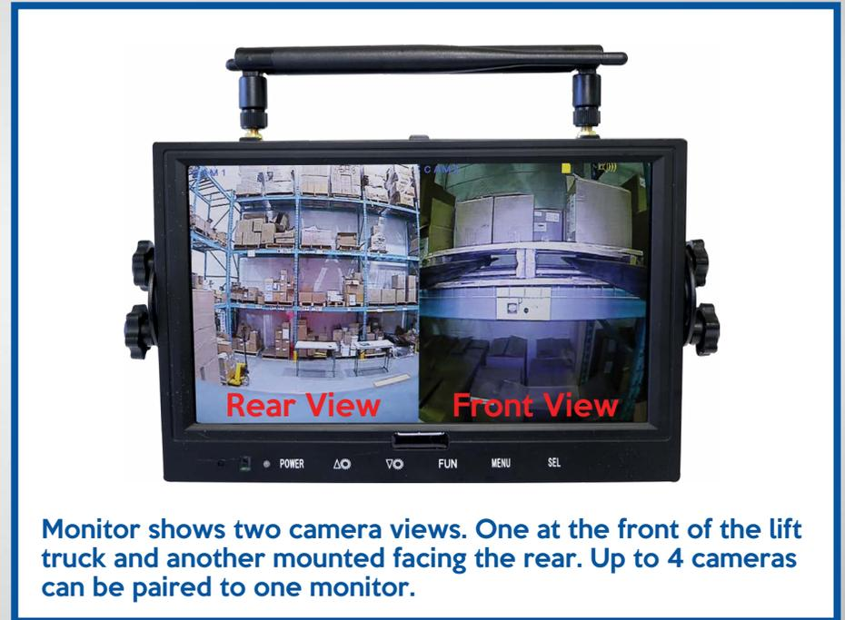
Monitor shows two camera views. One at the front of the lift truck and another mounted facing the rear. Up to 4 cameras can be paired to one monitor.
